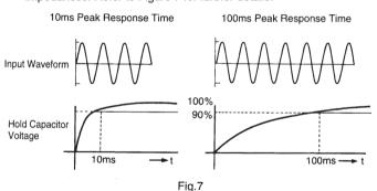
For instance, select the 10ms response time when measuring a surge current that will occur when a power supply device is switched on. The 100ms response time is recommended for measuring the starting current of a motor or similar equipment. A stable measurement can be made on the 100ms second response time setting as the peak hold circuit does not readily respond to the surge current.
