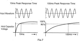
For instance, select the 10ms response time when measuring a surge current that will occur when a power supply device is switched on. The 100ms response time is recommended for measuring the starting current of a motor or similar equipment. A stable measurement can be made on the 100ms second response time setting as the peak hold circuit does not readily respond to the surge current.
